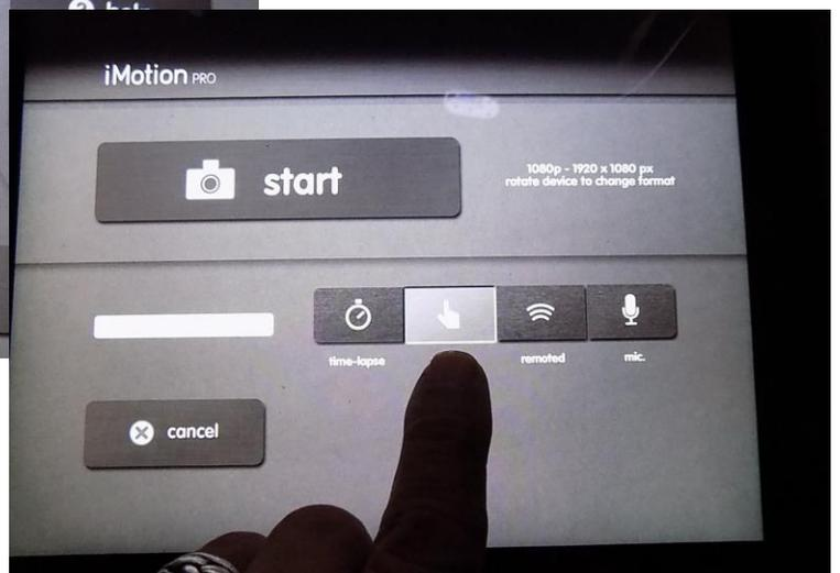
We are doing Stop Motion Animation so the first button, "Time-Lapse" is useless to use. We are only going to deal with "Manual", "Remoted" and "Mic" buttons. With the "Manual" setting you have to press the "Capture" button each time you want to capture a frame. This is okay but can lead to some chatter (shaking) between frames.
